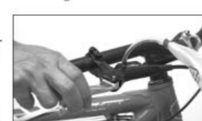
h-8. Depress the brake lever
