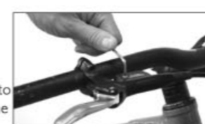
h-3. Remove the bolt that is inside of the reservoir tank
