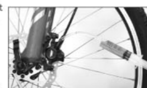
h-2. Attach the syringe to the outlet valve
