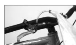
h-4. Attach a bag or a bottle to the tube
