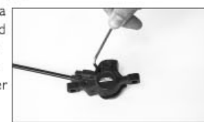
f-1. Unscrew pad retainer bolt
