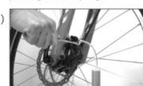
h-7. Tighten the caliper mounting bolts
