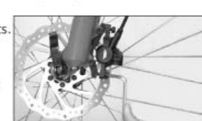
e-2. Attach the caliper to the adapter
