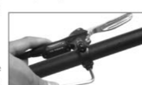
c1-2. Tighten the brake lever clamp
