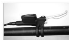
g-3. Position the lever parallel to ground
