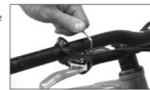
h-9. Tighten the bolt
