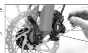
h-1. Remove the cover from outlet valve
