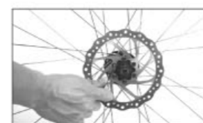
b-1. Mount the rotor to the hub
