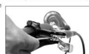
c1-3. Alter the reach adjustment
