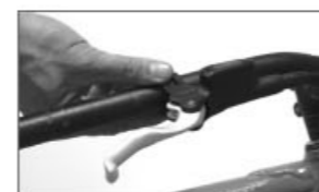
c-1. Slide lever onto handlebars
