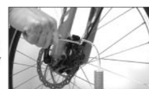
h-5. Open the outlet valve 1/4 turn.
