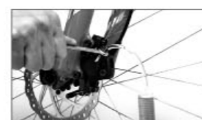
g-5. Open the outlet valve 1/4 turn.
