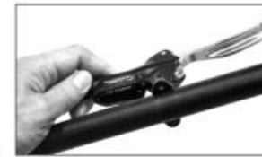
c1-1. Place the brake lever with the half clamp onto the handlebars
