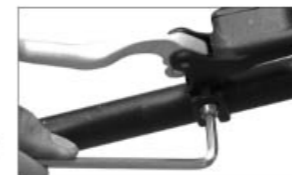
c-2. Tighten the brake lever clamp
