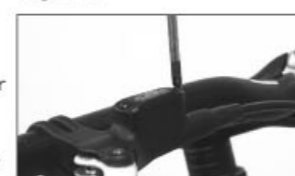
g-4. Remove the reservoir cover bolts
