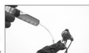
g-6. Fill the reservoir with oil
