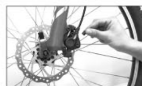
g-1. Remove the cover from the outlet valve
