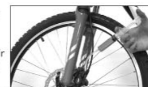
h-6. Fill the reservoir with oil by pushing on the syringe
