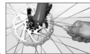
e-1. Mount the adapter to the frame/fork
